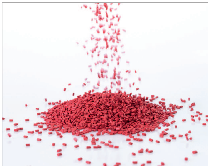
Fig. 2: Plastic granulate for injection molding or extrusion
